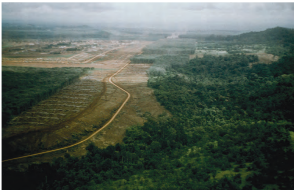
An aerial view of an anti-ambush clearing on each side of a road by Rome plows
